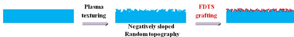
Figure 1. Two-step approach to obtain superamphiphobic surfaces via plasma-induced texturing and follow-up reaction with FDTS ( \text{Cl}_3\text{SiCH}_2\text{CH}_2\text{-C}_{10}\text{F}_{21} ).
